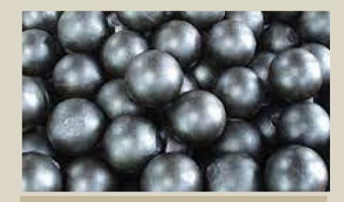
The proper selection of High Chrome media to minimize mineral surfaces contamination
